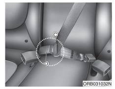
Pull and insert the tongue plate (C) into the open end of the buckle (D) until an audible "click" is heard, indicating the latch is locked.
