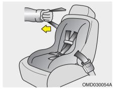
Pull the shoulder portion of the seat belt all the way out. When the shoulder portion of the seat belt is fully extended, it will shift the retractor to the "Automatic locking" (child restraint) mode.
