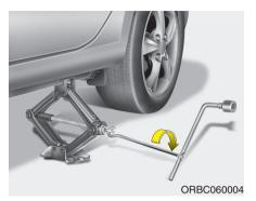
8. Insert the jack handle into the jack and turn it clockwise, raising the vehicle until the tire just clears the ground. This measurement is approximately 1.2 in (30 mm). Before removing the wheel lug nuts, make sure the vehicle is stable and that there is no chance for movement or slippage.
