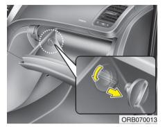
With the glove box open, remove the stoppers by turning them counterclockwise on both sides.
