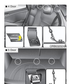
Securing a child restraint seat with "Tether Anchor" system
